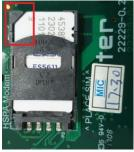
When placing the SAM(s), make sure that the SAM card is appropriately placed as shown in the image.
